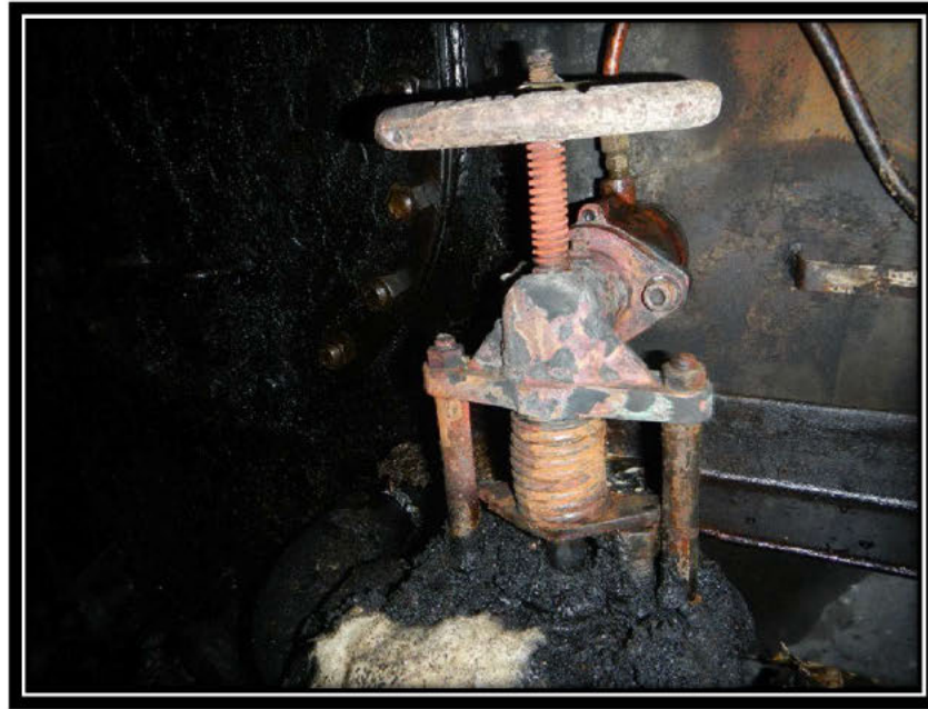
Figure 19; Post Casualty photo of Lube Oil Storage tank quick cut-off valve blocked open with bolt
