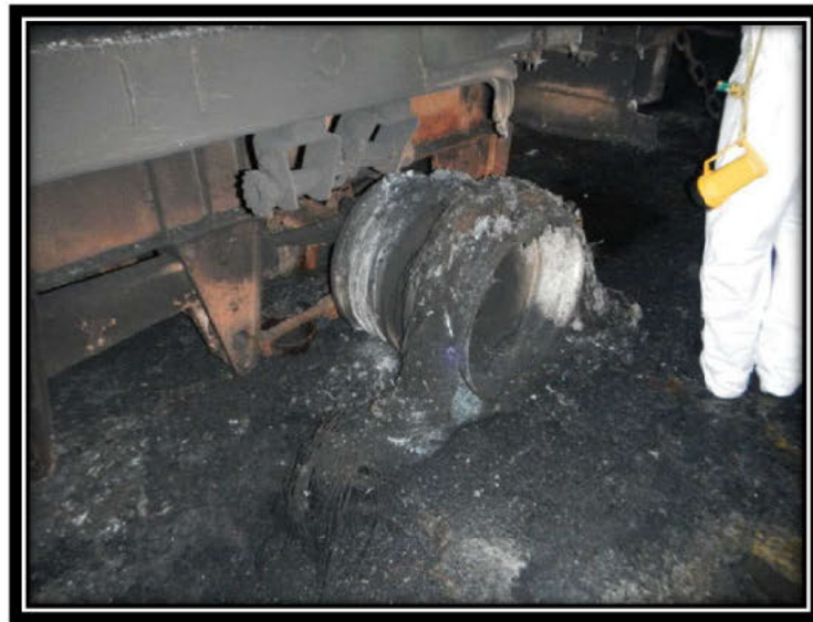
Figure 4; Post Casualty photo of container trailer wheels in Garage B directly over engine room (Secondary fire and source of explosions heard and reported by crew)
