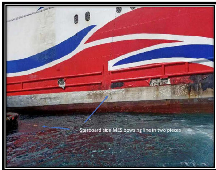
Figure 6; Post Casualty photo of Marine Evacuation System bowing line in two pieces.
