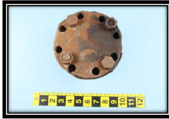
Figure 15; Post Casualty photo of Fuel supply line blank end examined in NTSB materials lab. (blank end view)
