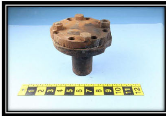
Figure 16; Post Casualty photo of Fuel supply line flange and blank end in NTSB materials lab. (profile)
