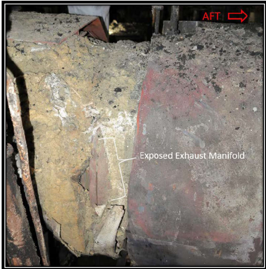
Figure 18; Post Casualty photo of STRB Main Engine with damaged thermal protection.
